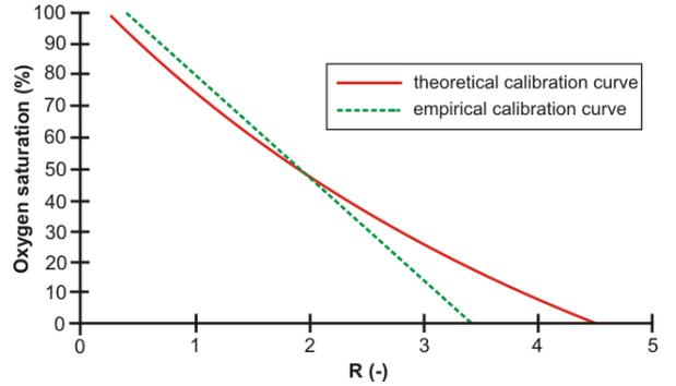
Fig. 5: Calibration curve
