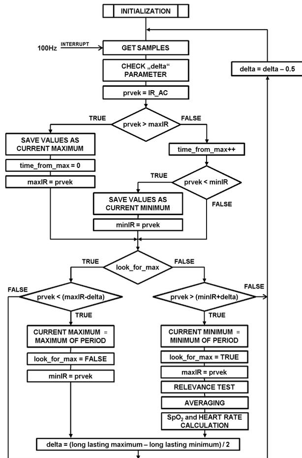
Fig. 3: Peak detector flow chart
