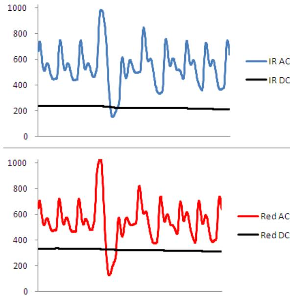
Fig. 4: Real oximetry signal with motion artifact
