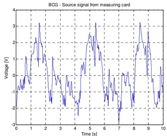
Fig. 4. RAW BCG from measuring card
