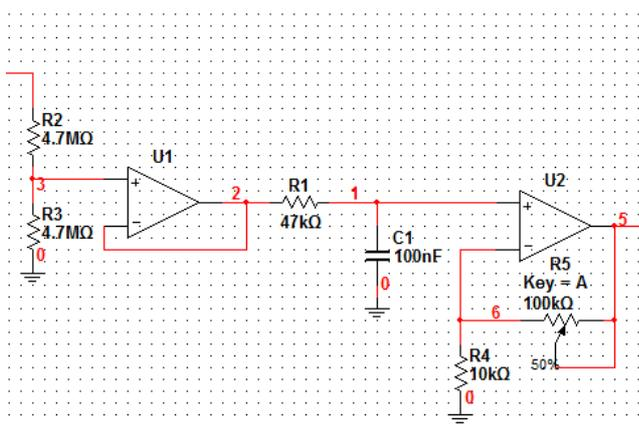
Fig. 2. Analog signal preprocessing circuit schema
