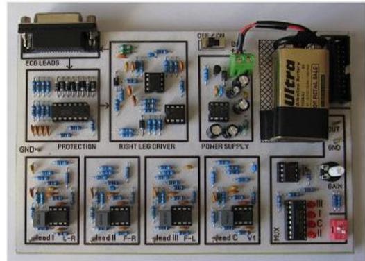
Fig. 3. The ECG signal measurement unit
