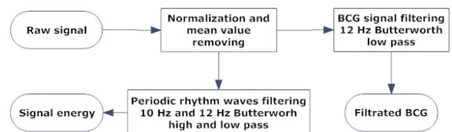
Fig. 5. BCG Digital signal processing block schema
